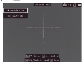
4. Press M, A, A and A to move the reticle position. The coordinate shows the current position of the reticle.
