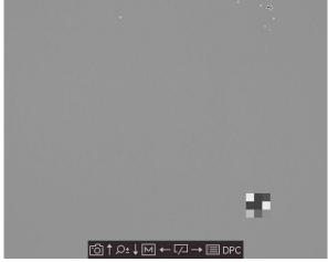
**Figure 3-3 Correct Defective Pixel**
