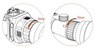
Figure 3-1 Adjust Focus Ring
