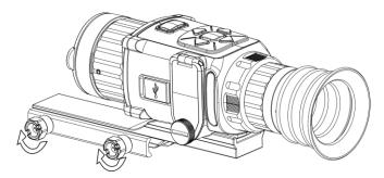
Figure 2-5 Secure the Device
