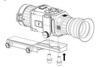
**Figure 2-4 Tighten Screws**
