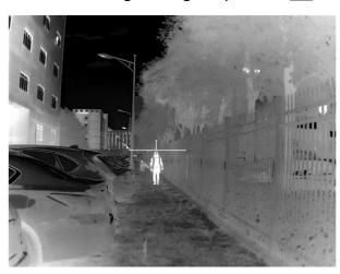
Figure 7-1 Set the Edge of Target Top
