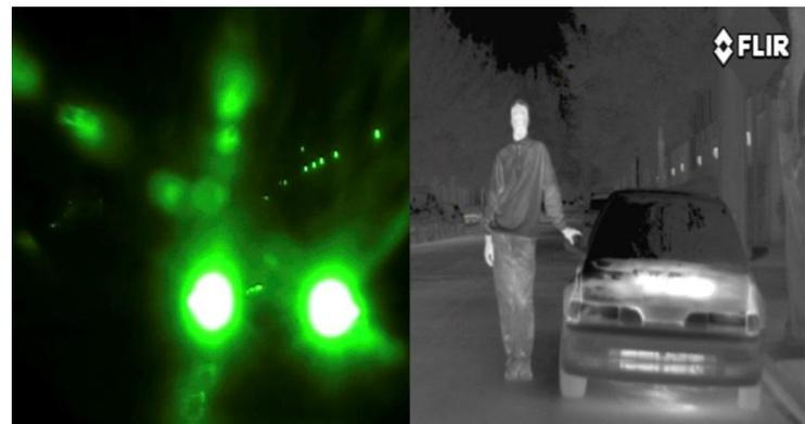
*Image intensification: image is saturated by looking directly to a light source.*
